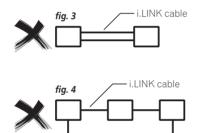
Another consideration when connecting i.LINK devices is the speed of the interface. At present there are three speeds; S100 (slowest), S200 and S400 (fastest). This amplifier uses the S400 type. Although you can use components with different speeds together, we recommend connecting slower-speed components at the edge of the network if possible (shown by the shaded boxes in figs. 1 and 2). This will keep the network free of bottlenecks.
